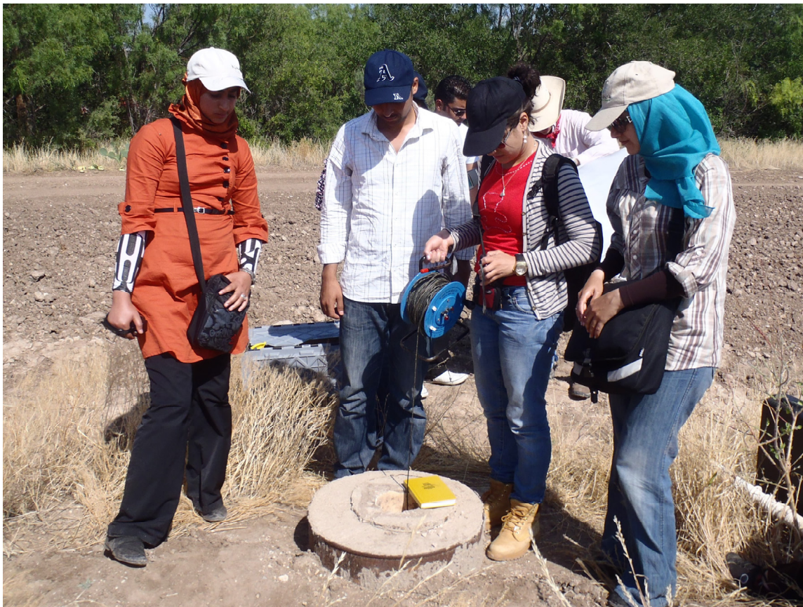
Figure 2. Field activities by Moroccan and Egyptian students around San Angelo, Texas: (a) gauging stream flow along Concho River; (b) measuring water level in monitoring well.
