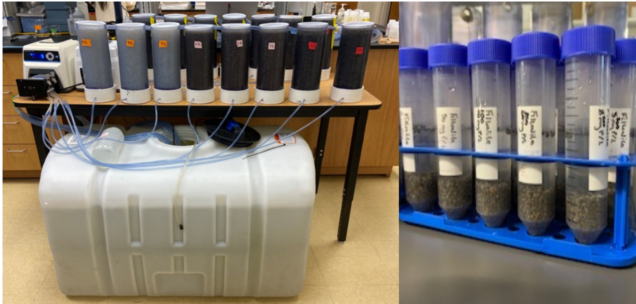
Figure 1. Experimental set-ups of flow-through column study (left) and sorption capacity batch study (right) in Coastal Ecological Engineering Lab at East Carolina University.
